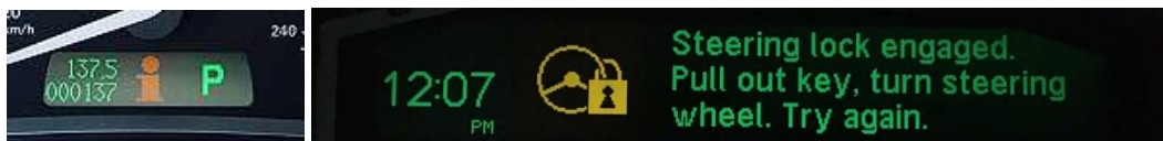
Example warning that will trigger eSID to go passive
