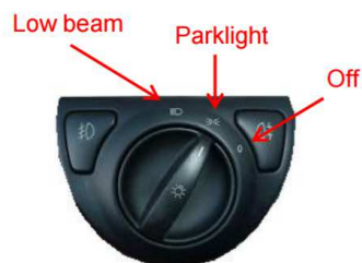
Main Light Switch
